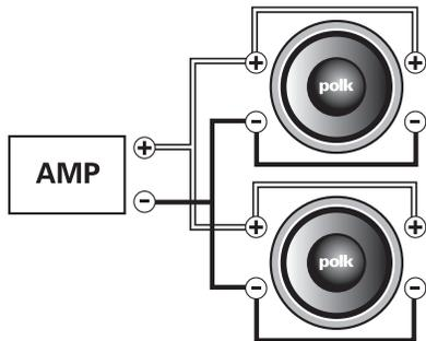
With coils and speakers wired in parallel, two dual 4 Ohm speakers will present a 1 Ohm load. (Not recommended unless amplifier is rated for 1 Ohm operation.)
