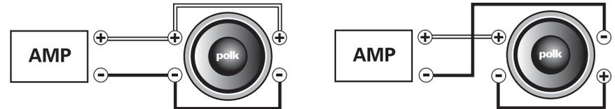
With coils in parallel, a dual 4 Ohm speaker will present a 2 Ohm load.
