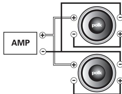
With the coils wired in series and the speakers wired in parallel, 2 dual 4 Ohm speakers will present a 4 Ohm load.
