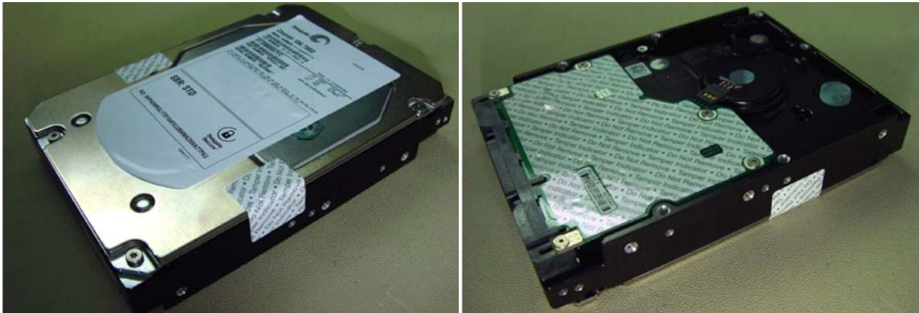
Figure 16. Example of FIPS tamper evidence labels.
