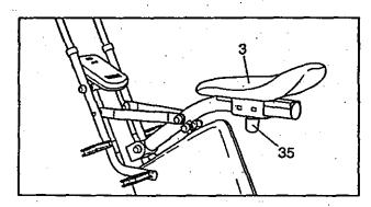
To adjust the position of the Seat (3), first turn the Seat Knob (35) to loosen it. Pull down the Seat Knob, move the Seat to the desired position, and release the Seat Knob. Slide the Seat back and forth slightly until the Seat Knob locks into place. Turn the Seat Knob to tighten it. Push on the Seat to make sure that the Seat Knob is engaged in one of the holes in the underside of the Seat Frame.
