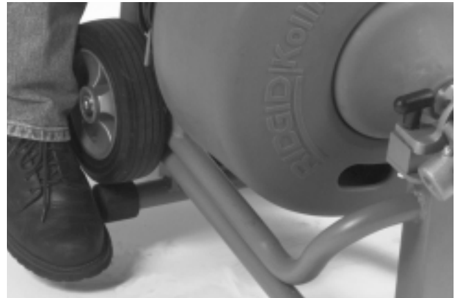
Figure 6 – Setting Kickstand Bar
