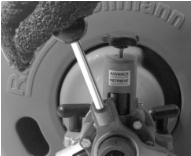
Figure 9 – Feed Lever Operation
