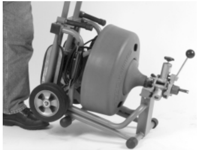
Figure 7 – Releasing Kickstand Bar
