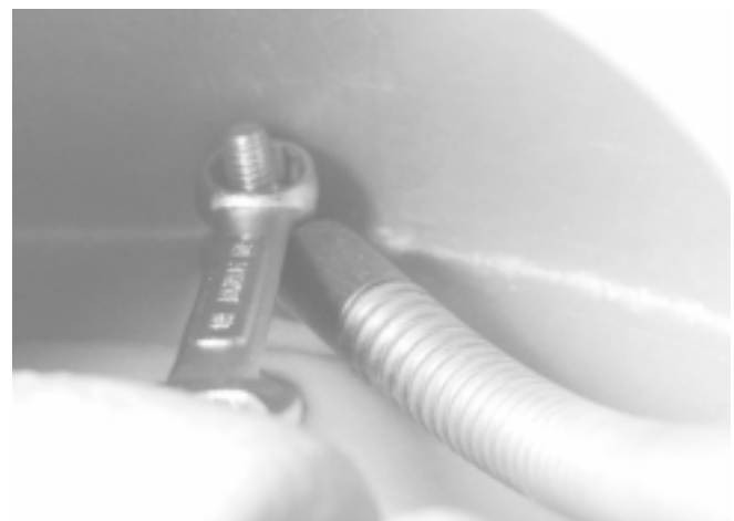
Figure 14 – Removing Pigtail Anchoring Bolt
