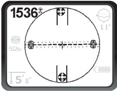
Figure 23 – Sonde Locate: Equator
