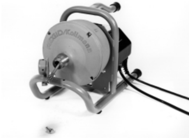
Figure 5 – Mounting Bracket Swung OPEN for Drum Access
