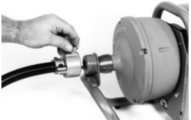
Figure 8 – Attaching Guide Hose to Mounting Bracket
