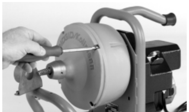
Figure 18 – Loosen 4 Drum Screws About 3 Full Turns But Do Not Remove
