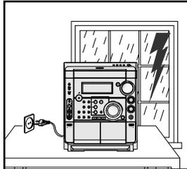
During thunderstorms, disconnect the main plug from the socket. Main voltage peaks due to lightning could damage the unit.
