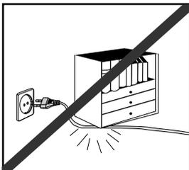
Do not place heavy items on the main lead. Main cable damage can lead to damage of the equipment (fire hazard) and can cause electric shock.
