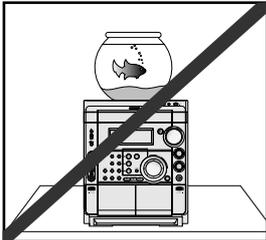
Do not place potted plants or vases on top of the unit. Moisture entering the unit could lead to dangerous electric shock and can cause equipment damage. In such events immediately disconnect the main plug from the socket.
