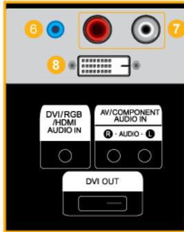
**6** *DVI/RGB/HDMI AUDIO IN (PC/DVI/HDMI Audio Connection Terminal (Input))*
