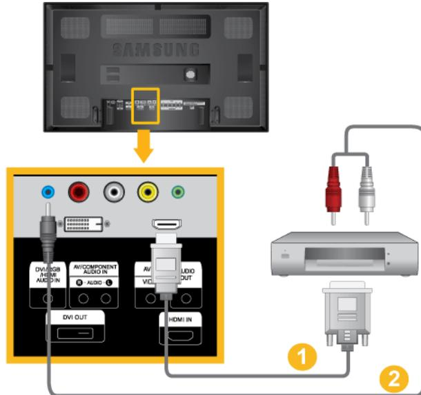
1. Connect the DVI output terminal of a digital output device to the [HDMI IN] terminal of the LCD Display using a DVI to HDMI cable.
