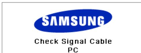
4. Turn off your LCD Display and reconnect the video cable; then turn on both your computer and the LCD Display
