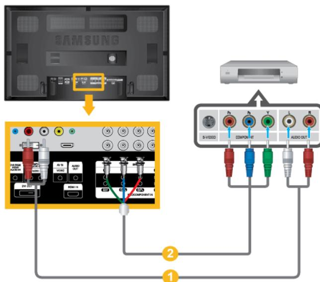
1. Connect a set of audio cables between the [AV/COMPONENT AUDIO IN [R-AUDIO-L]] on the LCD Display and the AUDIO OUT jacks on the DVD player.
