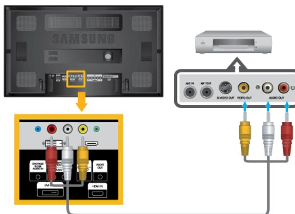
1. Connect an audio cable to the audio output port on the external device and [AV/COMPONENT AUDIO IN[R-AUDIO-L]] port on the monitor, and connect the video output port on the external device to the [AV IN [VIDEO]] port on the monitor.
