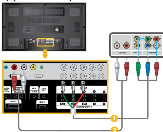
1. Connect a Component cable between the [BNC/COMPONENT IN [R/Y, G/P<sub>B</sub>, B/P<sub>R</sub>]] port on the LCD Display and the P<sub>R</sub>, Y, P<sub>B</sub> jacks on the Set Top Box.
