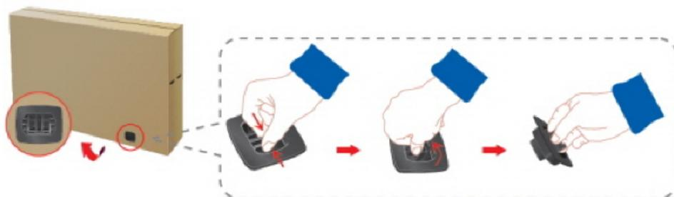
Remove the lock from the package box, as shown in the figure above.
