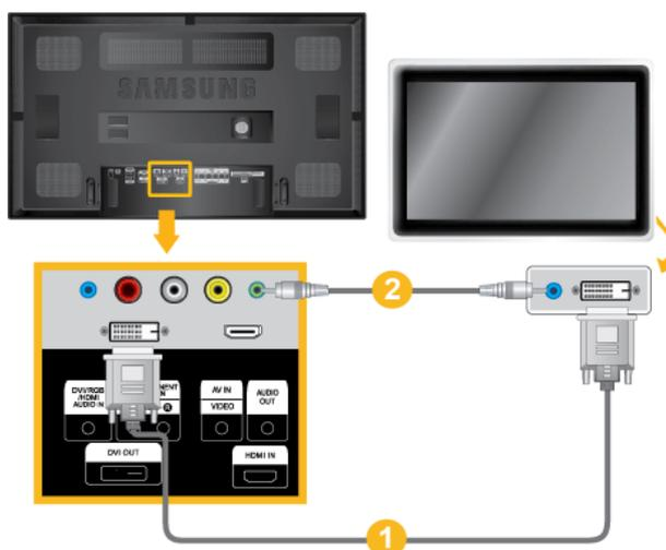
1. Connect between the [DVI OUT] port on the LCD Display and the input port on another monitor using a DVI cable.
