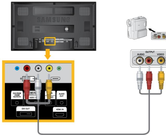
1. Locate the AV output jacks on the camcorder. They are usually found on the side or back of the camcorder. Connect a set of audio cables between the AUDIO OUTPUT jacks on the camcorder and the [AV/COMPONENT AUDIO IN [R-AUDIO-L]] on the LCD Display .
