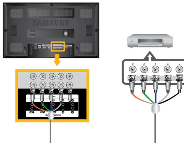
1. Connect the [BNC/COMPONENT IN [R/Y, G/P<sub>B</sub>, B/P<sub>R</sub>]] ports on the monitor to the BNC port on the external device using the BNC to BNC cable.
