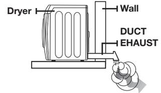
2. Use 4" diameter rigid metal duct. Tape all joints, including at the dryer. Never use lint-trapping screws.
