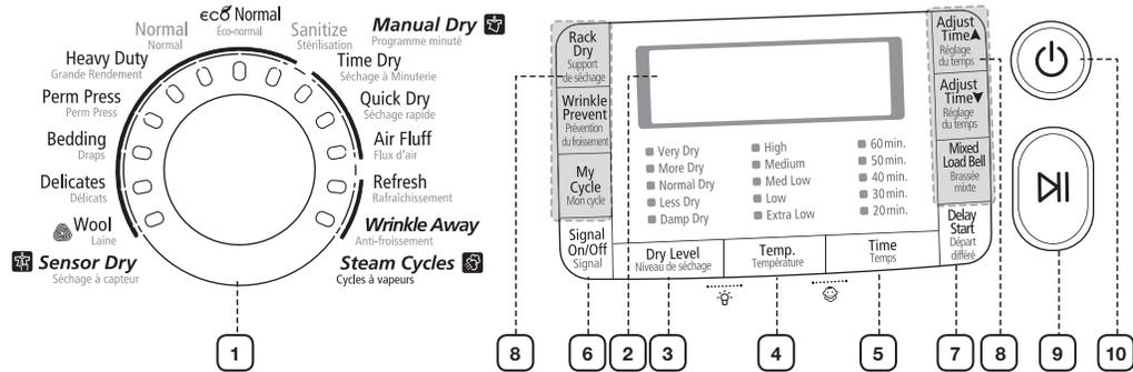
To select a cycle, rotate the Cycle Selector dial to the desired cycle.
