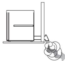
2. Use a 4" diameter rigid metal duct. Tape all joints, including at the dryer. Never use lint-trapping screws.
