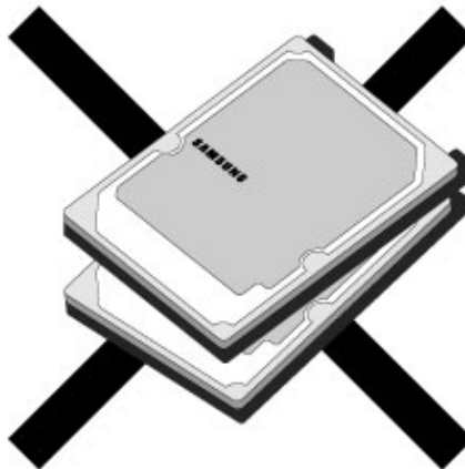
Fig. 9-3: HDD handling guide -Do Not Stack!
