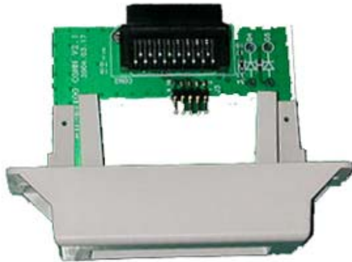
Bluetooth Connection PCB (RIF-BT10C)
