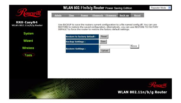
Backup Settings: This can save the Broadband router current configuration to a file named "config.bin" on your PC. You can also use the <Upload> button to restore the saved configuration to the Broadband router. Alternatively, you can use the "Restore to Factory Defaults" to force the Broadband router to perform a power reset and restore the original factory settings.
