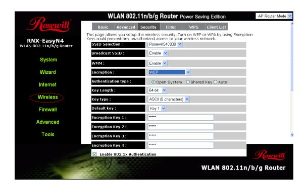
Authentication Type: There are two authentication types: "Open System" and "Shared Key". When you select "Open System", wireless stations can associate with this wireless router without WEP encryption. When you select "Shared Key", you should also setup a WEP key in the "Encryption" page. After this has been done, make sure the wireless clients that you want to connect to the device are also setup with the same encryption key.
