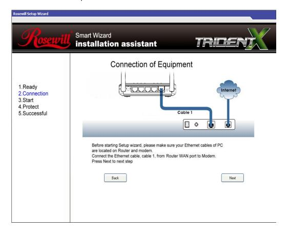
Check the MODEM and RNX-EASYN4 connection. It should be as shown below.
