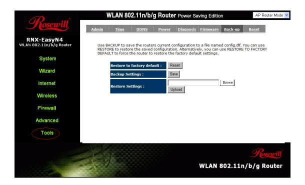
Backup Settings: This can save the Broadband router current configuration to a file named "config.bin" on your PC. You can also use the <Upload> button to restore the saved configuration to the Broadband router.
