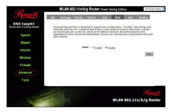
Enable/Disable UPnP: You can enable or Disable the UPnP feature here. After you enable the UPnP feature, all client systems that support UPnP, like Windows XP, can discover this router automatically and access the Internet through this router without having to configure anything. The NAT Traversal function provided by UPnP can let applications that support UPnP connect to the internet without having to configure the virtual server sections.
