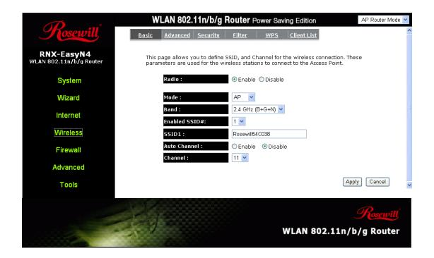
**Radio:** You can turn on/off wireless radio. If wireless Radio is off, you cannot associate with AP through wireless.
