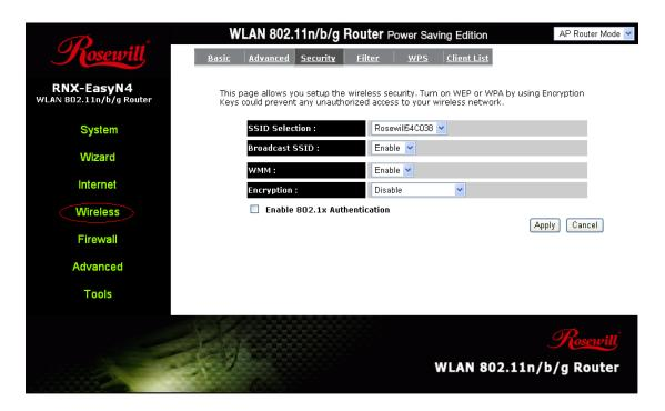
**ESSID Selection:** This broadband router support multiple ESSID, you could select and set up the wanted ESSID.
