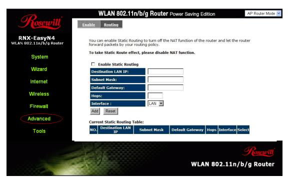
**Destination LAN IP:** Specify the destination LAN IP address of static routing rule.
