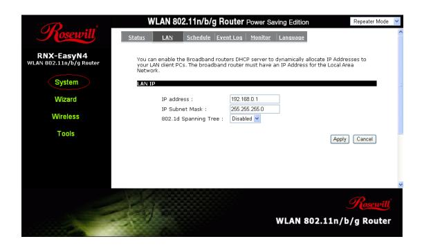
**IP address:** It is the router's LAN IP address (Your LAN clients default gateway IP address). It can be changed based on your own choice.
