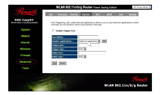
**Enable Trigger Port:** Enable or disable the Port Trigger function.
