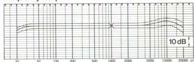
Standard frequency response with tolerance limits MKH 106 T, measuring distance 1 m.
