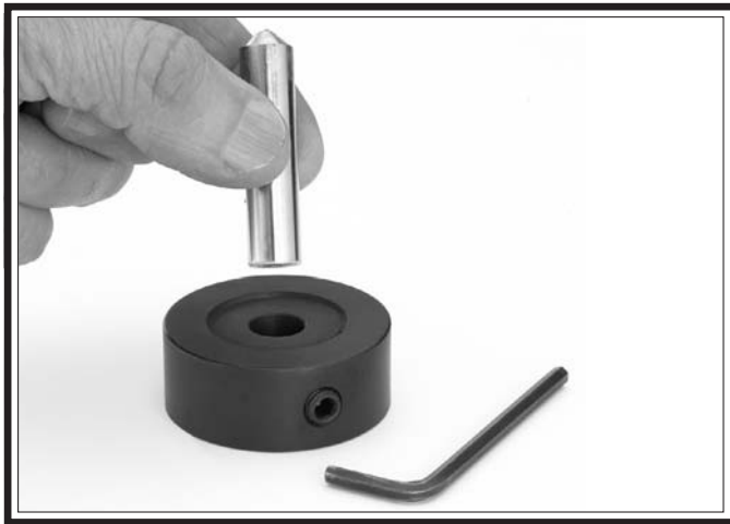
Figure 32. Dressing tool setup.
