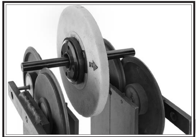
Figure 33. Wheel on balancing fixture.
