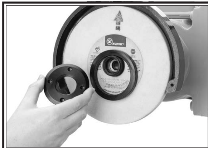
Figure 16. Exposing wheel spacer washer.
