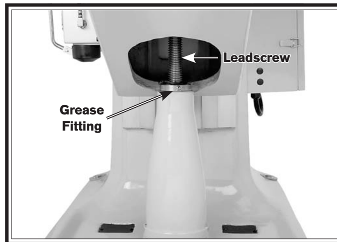
Figure 56. Table elevation leadscrew and grease fitting.
