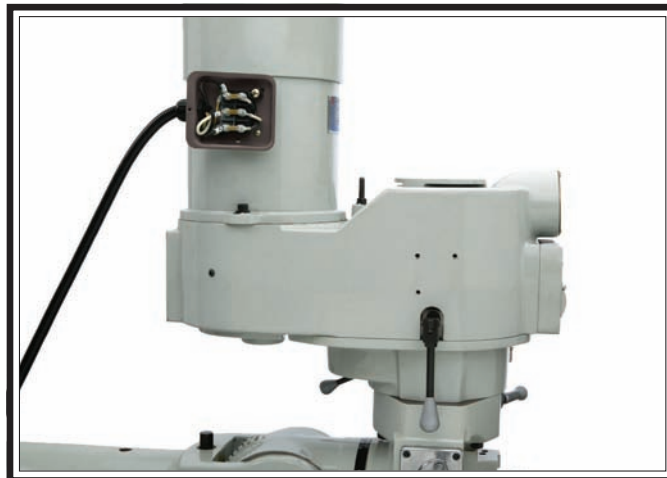
Figure 70. Motor junction box.
