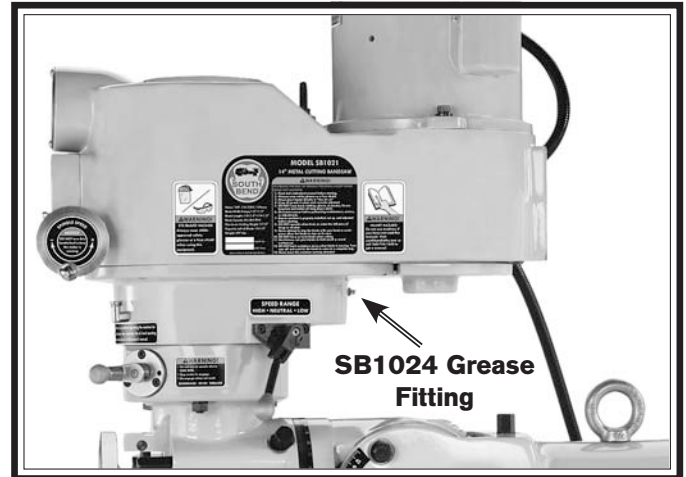
Figure 52. SB1024 headstock gearing grease fitting.
