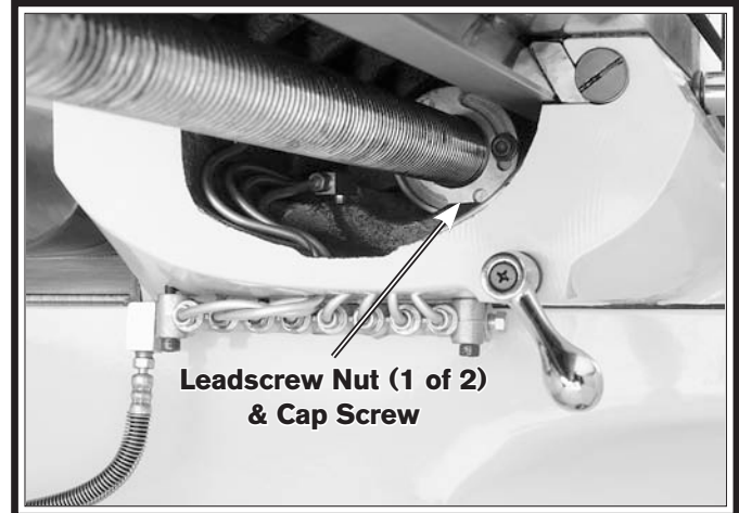
Figure 64. Longitudinal leadscrew nut and cap screw, as viewed from underneath the left side of the table.
