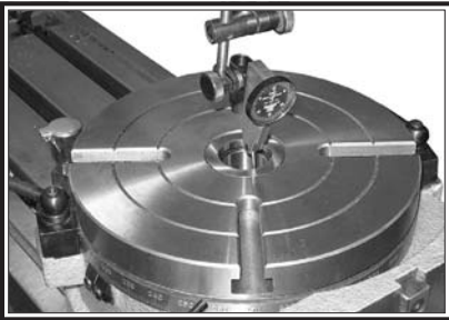
Figure 5. Example of using a test indicator to align a rotary table.
