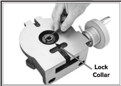
Figure 16. Loosening the spindle lock collar cap screw.
