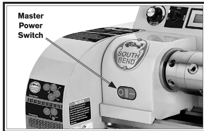
Figure 1. Master power switch location.
