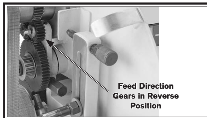
Figure 70. Feed direction gears in the left-hand threading position.
