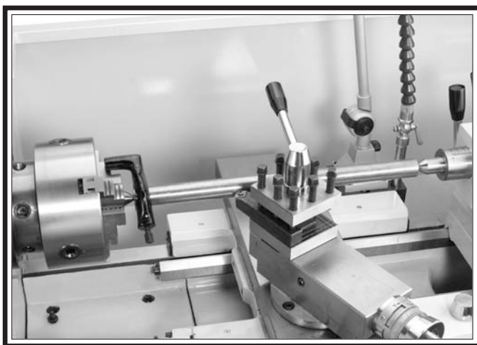
Figure 31. Example photo of stock mounted between the centers.
