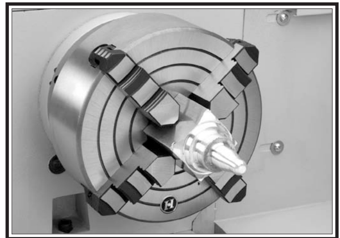
Figure 24. Example photo of non-cylindrical workpiece correctly mounted on the 4-jaw chuck.
