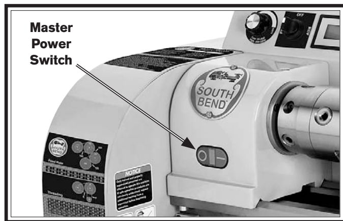
Figure 14. Master power switch location.
