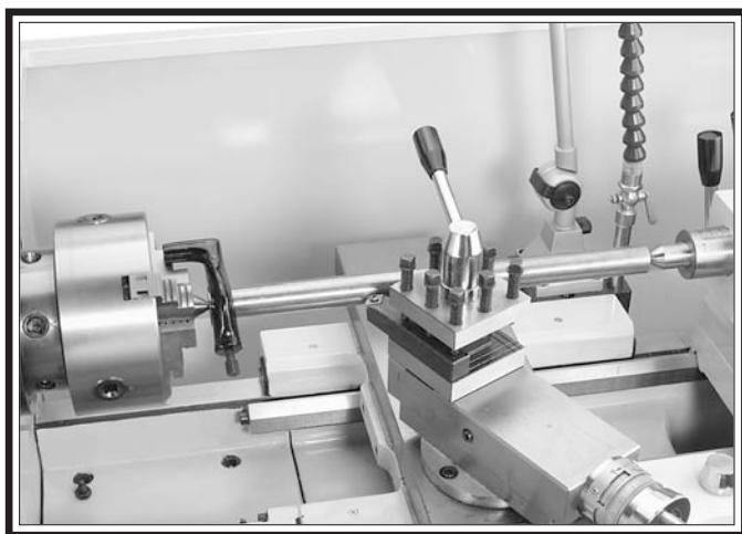
Figure 38. Example photo of a workpiece mounted between the centers.
