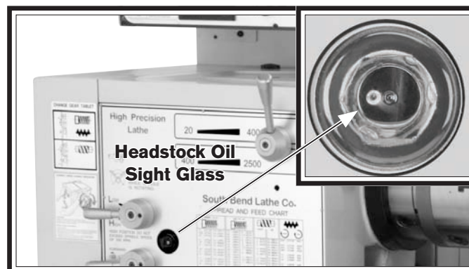
Figure 109. Location of the headstock oil sight glass.
