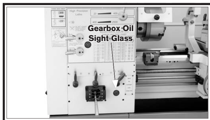
Figure 112. Gearbox sight glass location.
