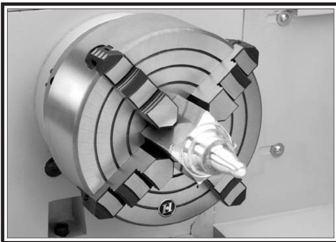
Figure 36. Example photo of non-cylindrical workpiece correctly mounted on the 4-jaw chuck.
