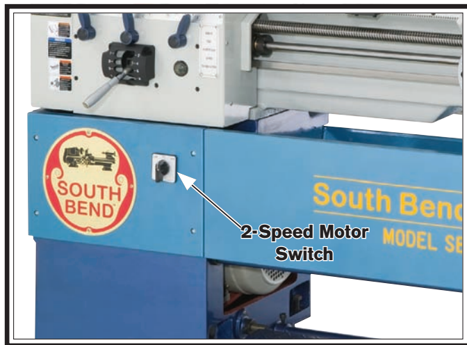
Figure 153. 2-Speed motor switch.
