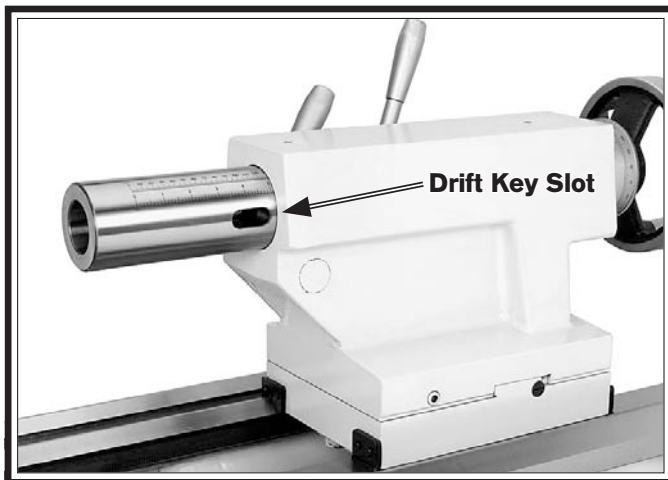
Figure 59. Drift key slot in the side of the quill.
