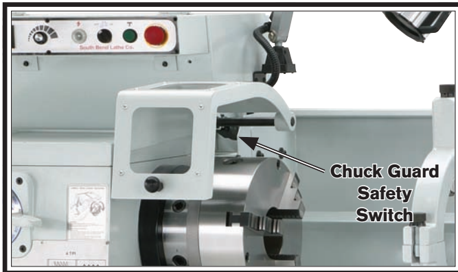
Figure 150. Chuck guard limit switch.
