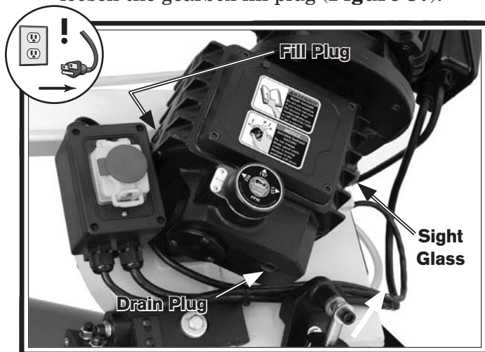
Figure 37. Gear box lubrication.
