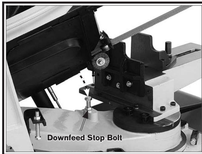
Figure 11. Adjusting downfeed stop bolt.
