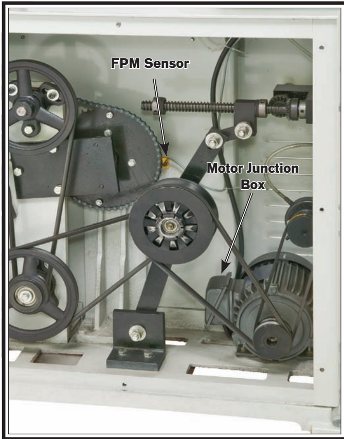
Figure 53. Motor and FPM sensor.
