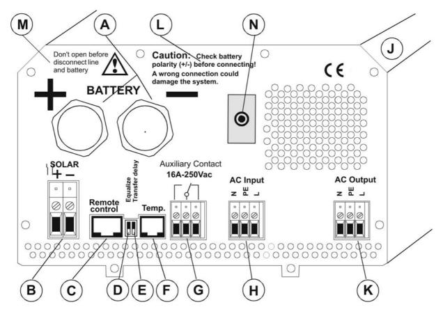
A Battery +/- Battery cable (already installed)
