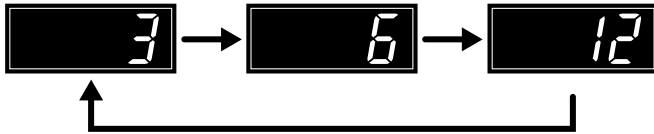
fig1. FADER PITCH SPAN SELECT SWITCH
