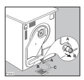
If the appliance is stacked on the washing machine, the condensed water can be discharged through the hose as shown in figure, but take into account that the hose must be pointed downwards.
