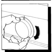
Following indications given in the drying times chart, turn the selector dial clockwise on the 55 mins setting. The dryer starts operating.
