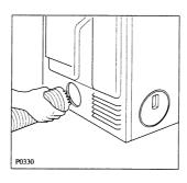
Remove the collar by pulling it out of the vent outlet. Screw the collar to the vent hose.
