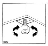
Level the tumble dryer into place by screwing or unscrewing the front feet as required.
