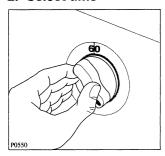
Turn the selector dial clockwise to the required minute setting.
