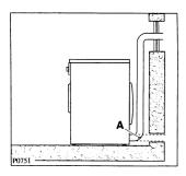
Connect the other end of the hose to an opening in a door or window. Fit a suitable shield or point the hose downwards to prevent any rain water and wind from getting in.
