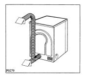
The vent hose must not contain more than two bends when it is placed in position for operation.
