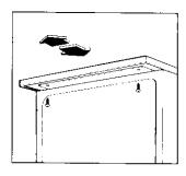
You can move the worktop forward or backward by 25 mm in order to align the machine with other kitchen units.
