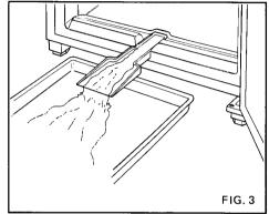
5. After defrosting, clean and dry the interior as explained under "Cleaning" and remove the plastic scraper. Switch on, replace any frozen food and close the door.
