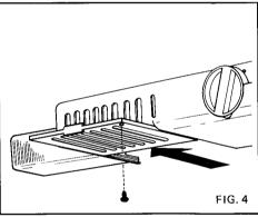
To replace the light cover slide it into its original position and replace screw.
