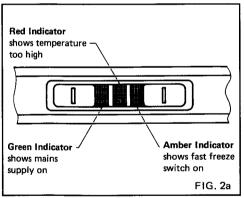
Operate the fast freeze switch to uncover the amber indicator (fig. 2a) and set the fridge thermostat knob at 4. The freezer/ fridge should then be left for a number of hours before use.
