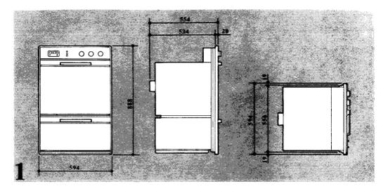
Dimensions of the recess for building into a tall kitchen unit (column)
