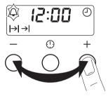
Press + or - to set the necessary clock function.
