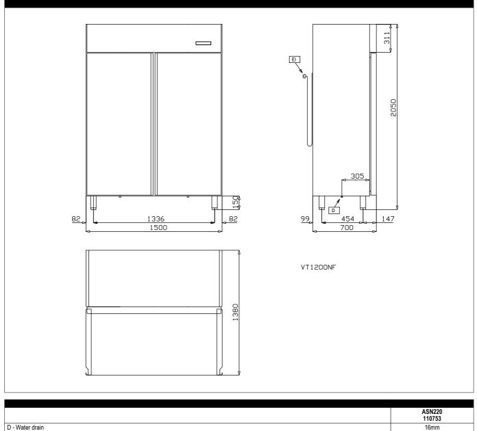
D - Water drain EI - Electrical connection
