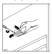
Unscrew the light cover and then pull it outward toward the middle of the cabinet. Unscrew the bulb and replace it with a new 15 watt bulb (available from your nearest Service Force Centre).
