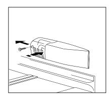
Unscrew the light cover and then pull it outward toward the middle of the cabinet. Unscrew the bulb and replace it with a new 25 watt bulb (available from your nearest Service Force Centre).
