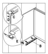
Snap vent grill (B) and hinge cover (E) into position.
