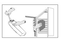
Disconnect the appliance from electricity supply. Clean out the drip channel inside the fridge at regular intervals and ensure that the drip channel is clear at all times. If blocked carefully clear using a piece of flexible curtain wire inserted into the drain outlet to remove the blockage.
