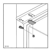
Position the runners (H) at the top and bottom of the inside of the kitchen unit as shown in the figure and mark the position of the external holes.
