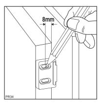
Remove the little plates and make the holes with a diam. of 2 mm. Replace the little plates over the runners and screw in the screws provided (3,5x16 mm). For the alignement of the kitchen unit door, if necessary, use the clearance size of the slotted holes. At the end of the procedure, check that the doors of the appliance and the kitchen unit open properly.
