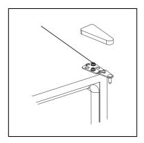
6. Unscrew the upper hinge and remove it, then lift the door and put it on a padded surface to prevent it be scratched. Put the upper hinge and the screws in a safe place.
