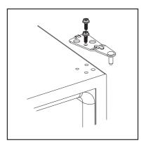
7. Pull out the cover-slip using a flat object, move it to right side and insert into the uncovered holes.
