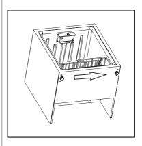
13. Fix the lower hinge with screws on the other side.
