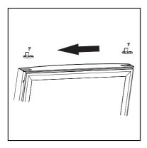
10. Unscrew and remove the lower hinge pin and install it to other hole.
