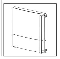
5. Lay down the appliance back side down and remove the upper hinge cap.
