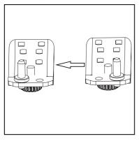
11. Unscrew the screws that fix the lower hinge and take the lower hinge with foot off.
