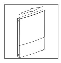
9. Rotate the door, then unscrew the screw and transfer the stopper to other side. Then securely fix the stopper with screw.
