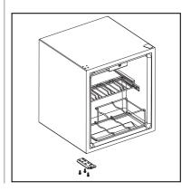
14. Put the door on the lower hinge. Keep the door closing the cabinet and put the upper hinge into the hinge hole. The right and left side of the door must aline with the sides of the cabinet. Then securely fix the upper hinge.
