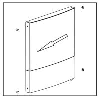
Fix the handle on the left side, insert the plastic covers that can be found in the bag for use instruction.
