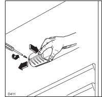
**2.** Replace the light cover by sliding it into its original position and replacing the screw.
