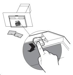
Position the new charcoal filter in the position marked and while holding the filter replace the fixing hooks as illustrated.
