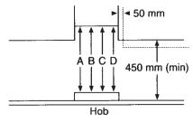
A: Built-in Electric Hob: 650mm minimum clearance
