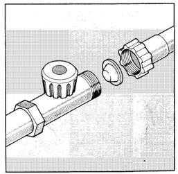
The other end of the hose which is connected to the appliance can be turned in any direction by first loosening the ring nut.
