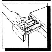
Pour the washing powder into compartment lacksquare, the main wash compartment.
