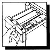
The compartment marked with the symbol !!! is for the prewash powder (if required by the programme).
