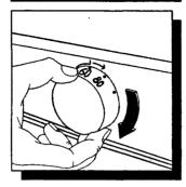
Following indications given in the drying times chart, turn the selector dial clockwise on the 60 mins setting of the blue section (Low Temperature Range).
