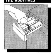
Pour the softener, if required, into the compartment marked \$\mathbf{S}\$ ; do not exceed the MAX level.
