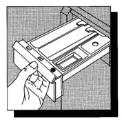
The compartment marked with the symbol  $\coprod$  is for the prewash powder (if required by the programme).
