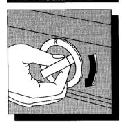
Press and turn the programme dial **clockwise** until letter **K** on the dial coincides with the red marker line.
