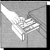
Pour the washing powder into compartment  $\coprod$ , the main wash compartment.
