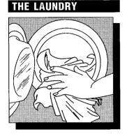
Open the door by pulling the catch outward. Load the items to be washed one at a time and close the door.
