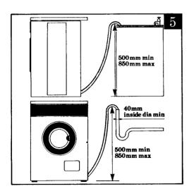
Finally, make sure that with the machine in position, the drain hose is not obstructed, blocked or bent so sharply that water cannot flow freely. The electrical connections Warning: THIS APPLIANCE MUST BE EARTHED
