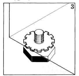
After levelling the machine, lock the feet by means of the securing ring nuts. Some vibration is inevitable, especially if mounted on a wooden floor, so make sure there is a gap of at least 12mm (1/2") between the machine and any walls, furniture and so on.
