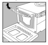
Remove the polystyrene base. Set the machine upright and unscrew the remaining rear screw. Slide out the relevant pin. Fill all the holes with the plastic plugs supplied with the instruction booklet.
