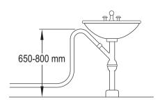
The drain hose can be connected directly into the pipe (e.g. beneath a washtub or sink), above the water trap. The drain hose must be arranged so that some part of it's length is routed up to a level corresponding to the top edge of the tub and fixed in place there.
