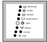
To select **Drain**, press the SKIP button three times, the **wash - rinses - spin** LED,s go out.
