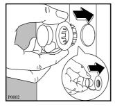
Slide out the 3 plastic spacers and plug the 3 holes with the 3 plastic plugs which you can find at the back of the machine.
