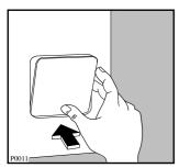
Open the filter door and place a container underneath to catch any spillage. If the filter is blocked and the machine is unable to drain you will need to drain the water manually from the machine at this stage. To do this, unhook the drain hose from the
