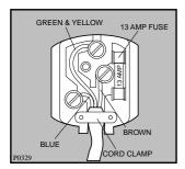
Connect the green and yellow (earth) wire to the terminal in the plug which is marked with the letter «E» or the earth symbol  $\bot$  or coloured green and yellow.
