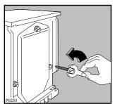
Using a spanner unscrew and remove the rear right bolt. Lay the machine gently on its back, making sure that the hoses are not squashed.
